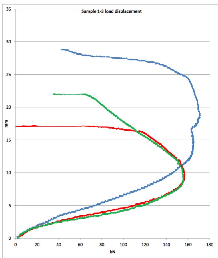
For an average 150kN failure, adopting a safety factor of 3 would give a safe working load of 50kN.
